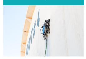
Examine and test water tanks without the need for service interruption. The robot operates autonomously to assess tank condition and detect potential issues.
